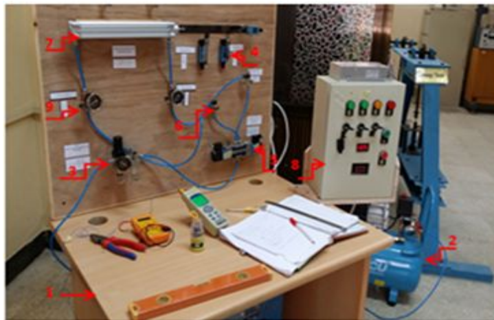
Figure 4: the Employed Electro Pneumatic Position System.
